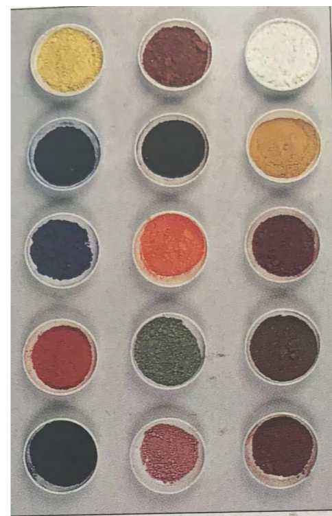
A selection of pigments prepared by Patrick Baty for the Building of Bath Museum including White Lead, Ochres, Umbers, Burnt Sienna, Venetian Red, Terte Verde, Potter's Pink, Prussian Blue, Vermilion and indigo. (The Georgian Group)
